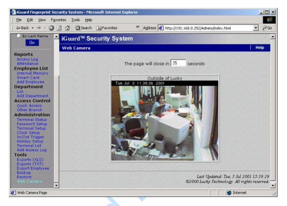
Currently the only supported web camera is *Axis 2100 Network Camera* from *Axis Communications* and the *JVC camera* from *JVC.*<sup>1</sup> Up to four Web Cameras can be supported at the same time and shown in the same page.
